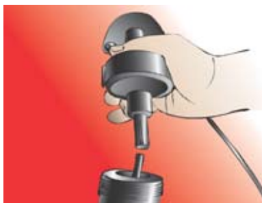
Screw on the new upper hinge with sensor.
