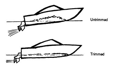
A good way to reveal your boats optimum attitude is to conduct a test by running lightly loaded at full speed in flat water. (This should be done in an open, no traffic area.) You will know your boats ideal attitude by observing the bow in relation to the horizon, reduced bow spray, and diminished wake.
