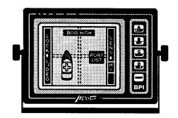
**Trimdicator** ®: Trimdicators are electronic trim tab position indicators. They display the position of each trim tab in degrees and percent of deflection. The Trimdicator features two electronic LCD / LED displays (one port - one starboard). The Trimdicators share the same CPU as the ATC system and can therefore be added at a reduced cost over the complete kit.
