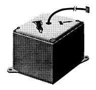
**Attitude Sensor-** The Attitude Sensor detects your boat's deviation from the "zero point" you store in memory and sends a continuous signal to the Central Processing Unit.
