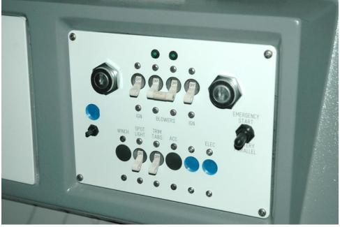
These are the panel indicators. For 12v you have to wire a 400 ohm ¼ watt current limiting resistor in series with each one. They are quite bright. Maybe an 800 ohm would be better. The originals were very dim.
