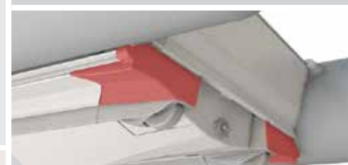
Built in trim tabs promote earlier planing and incorporate launching wheels
