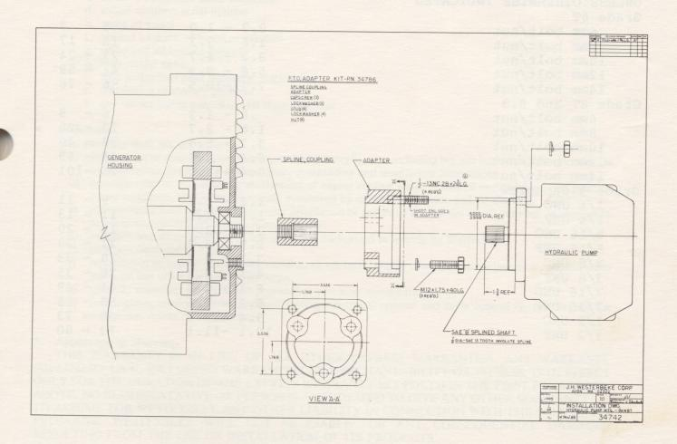
NOTE: Provisions should be made to prevent the P.T.O. device from overloading the generator engine, i.e., pressure relief valve.
