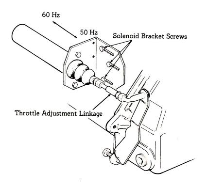
Solenoid and Throttle with Linkage
