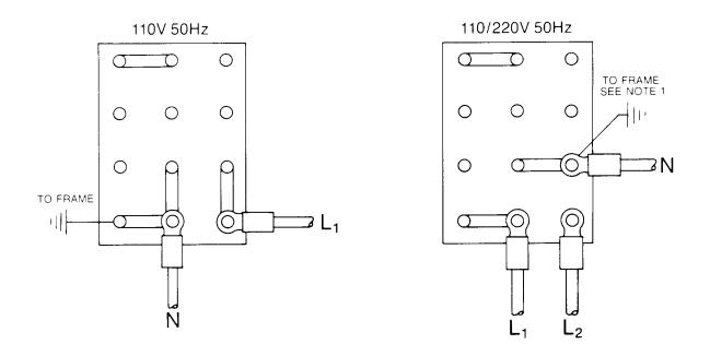
NOTE: The frame ground wire must be moved when changing from 110 volts 50 Hertz to 110/220 volts 50 Hertz.
