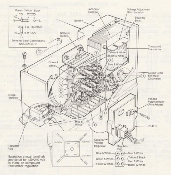
Under no circumstances attempt to increase the No Load voltage by increasing the gap between the laminated steel bar and the transformer core without the use of shims. Magnetic forces created within the transformer during generator operation may close the air gap and reduce No Load voltage output.
