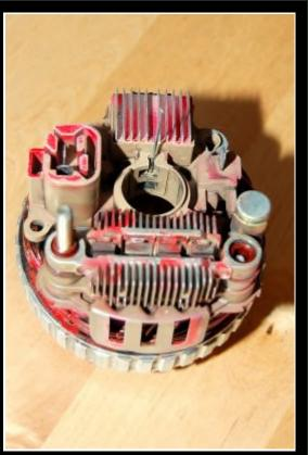
In this photo you'll notice a 2" long brad nail stuck into a tiny hole next to the brushes. This is how you retain the brushes to re-install the rotor. I found this 2" brad nail to be the perfect tool to retain these brushes.
