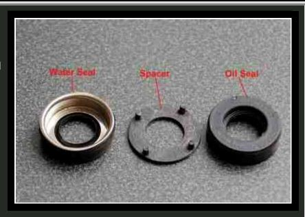
spacer sits, and is captive, right over the weep hole to let a leak drain and become visible and detectable.
