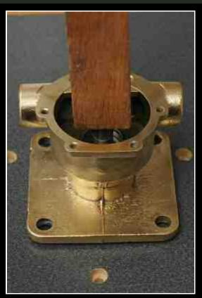
alternative method. If you are of a mechanical mind set and own a lead or brass hammer then it would be OK to tap directly on the shaft as brass and lead are softer than the shaft material. If you do not own a soft metal hammer simply insert a block of wood such as Maple, Oak or Teak, as I have done here, and tap on the wood with a regular hammer.
