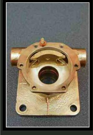
The first thing I re-installed was the pump cam. Be sure to use the small copper crush washer that came with the rebuild kit or it will leak out of the screw hole..
