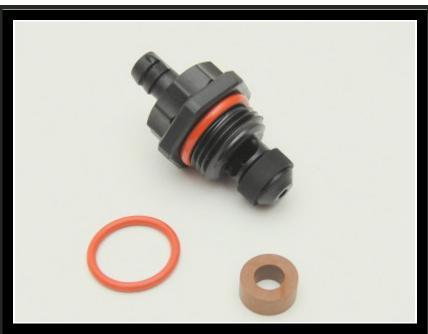
This is the drain plug / pet cock assembly from the bottom of the bowl. Use a wrench on the nut closest to the polycarbonate bowl to back it out, righty tighty, lefty loosey. The nut closest to the hose barb is the nut that opens and closes this petcock and is
