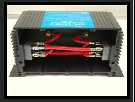
going to the gold plated studs. This is where your green grounding wire would be cut and connected to. Inside we can see the two diodes which allow current to flow in both directions but at the same time blocking voltages below 1.0 - 1.2V.
