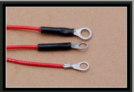
The black shrink was only used for photographic contrast. Normally I would use red, as shown in the last photo, so as not to insinuate this red wire is a negative conductor.
