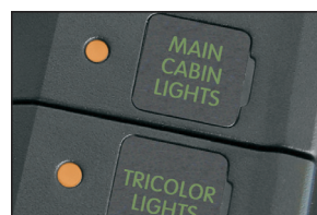
Circuit status LEDs and backlit labels aid low-light readability
