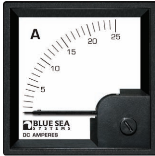
1052 Ammeter 0-25A Shunt type: Internal Connection: 2 wire - no other power required Weight: 0.13 lb (0.15 kg)
