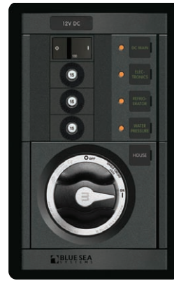
1402 • Backlit circuit labels • 3 Unswitched 24-hour circuits • ON indicating LEDs • 1 C-Series Flat Rocker Circuit Breaker (MAIN 100A) • 3 Push Button Reset-Only Circuit Breakers (BRANCH 15A) • Battery Switch: m-Series, 6006200
