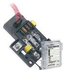
SafetyHub 100 Fuse Block—Holds 3 MIDI® or AMI® and 4 ATO® or ATC® Fuses Vmxo Maximum Voltage: 12V DC Imxo Maximum Amperage per block: 300A DC MIDI® or AMI® Fuse Block— Imxo Maximum Amperage per circuit: 200A DC ATO® or ATC® Fuse Block— Imxo Maximum Amperage per circuit: 30A DC Imxo Maximum Amperage per block: 50A DC
