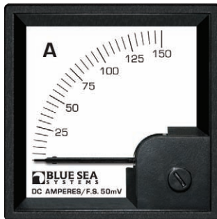
1055 Ammeter 0-150A Shunt type: External—50 mV at full scale Connection: 2 wire from shunt - no other power required Weight: 0.53 lb (0.24 kg)
