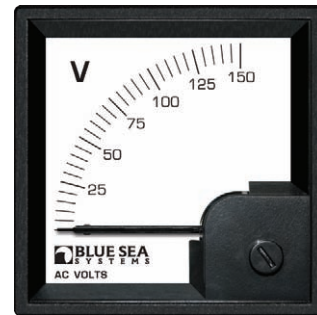
1056 Voltmeter 0-150V Connection: 2 wire to AC hot and neutral Weight: 0.33 lb (0.15 kg)
