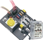
SafetyHub 250 Fuse Block with Remote Battery Switch—Holds 3 MIDI® or AMI® and 4 ATO® or ATC® Fuses Vmxo Maximum Voltage: 12V DC Imxo Maximum Amperage: 240A DC MIDI® or AMI® Fuse Block— Imxo Maximum Amperage per circuit: 200A DC ATO® or ATC® Fuse Block— Imxo Maximum Amperage per circuit: 20A DC Imxo Maximum Amperage per block: 50A DC
