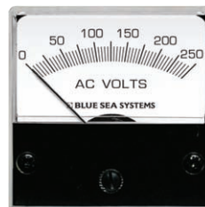
8245 Micro Voltmeter 0-250V AC Connection: 2 wire to AC hot and neutral Meter Face Size: 2" Weight: 0.26 lb (0.12 kg)
