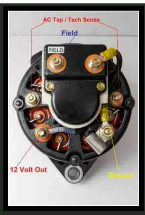
output stud gets wired directly to the positive side of your boats electrical system. I recommend wiring this directly to a battery, such as the house bank, so you can't fry the alternator diodes by turning off the battery switch when the motor is running.
