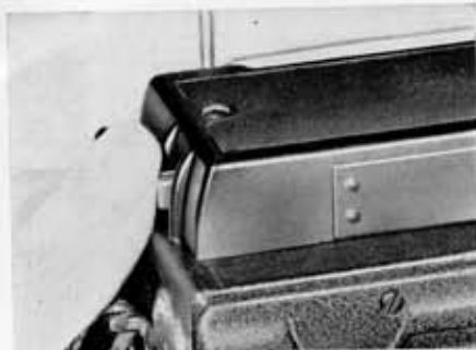
7. The Rangelite in the Graphic Rangefinder is operated by the push-button on the left of the rangefinder housing. Two beams of light are projected through the rangefinder windows.
