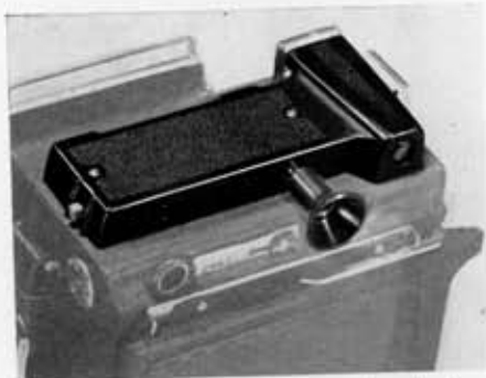
1. Back view of Graphic Rangefinder showing: (right) Optical Viewfinder; (center) Rangescope magnifier; (left) Rangelite switch.
