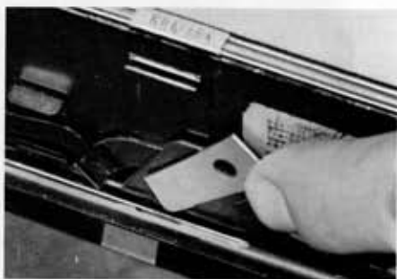
4. Smaller end of cam is dropped into slotted tube first. Cam is inserted with the numbered side up, facing top of camera.
