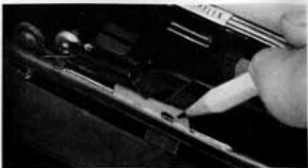
6. Pencil points to cam inserted in slot and in position to couple the lens to the rangefinder. Final step is to release hinged cover.
