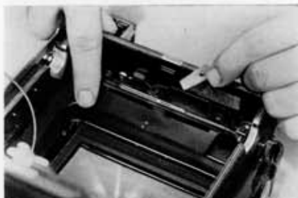
3. Hinged cover is held open as rangefinder cam is held ready to be placed in the slotted tube. Each lens has its own cam.
