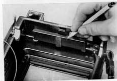
2. Hinged cover of Graphic Rangefinder, under the top of Speed Graphic Camera. Cover is pulled down to insert the cams that couple the interchangeable lenses to the rangefinder.
