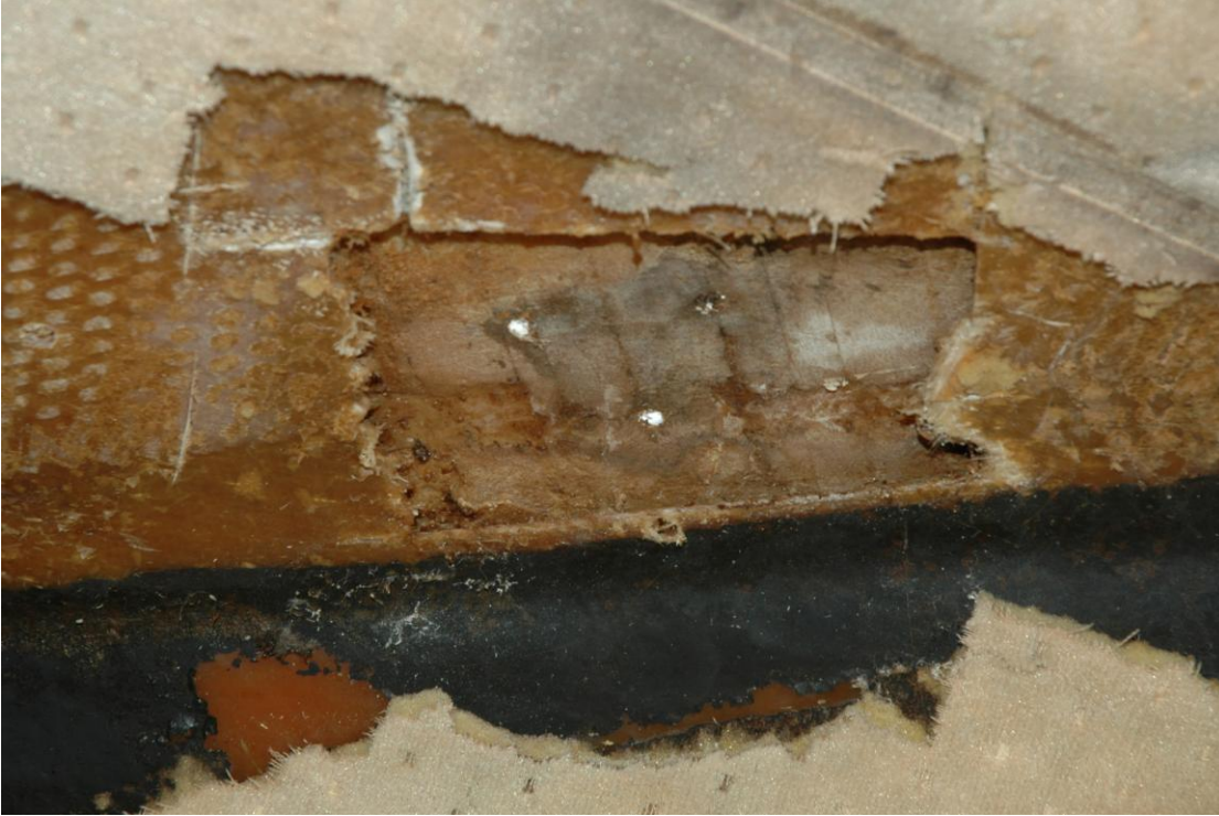
Figure 10 Stanctions have backing plates and nuts and washers below.
