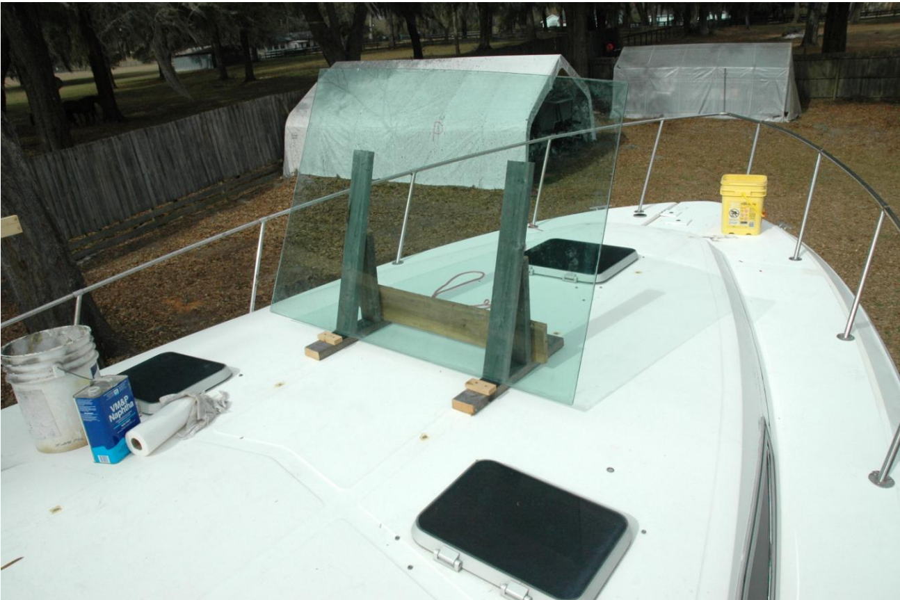
Figure 15 Glass is really big. NEVER lay flat! Always on edge!
