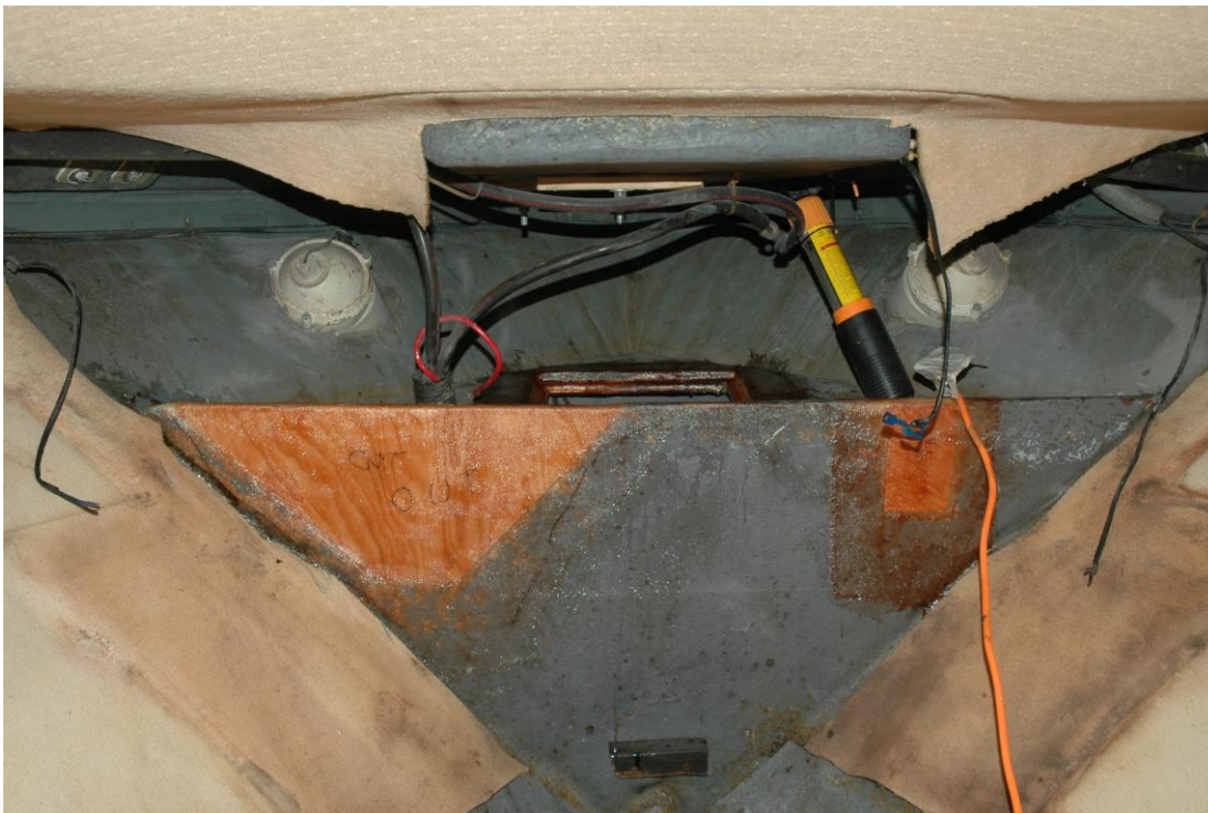
Figure 6 Water from above rotted out the bulkhead
