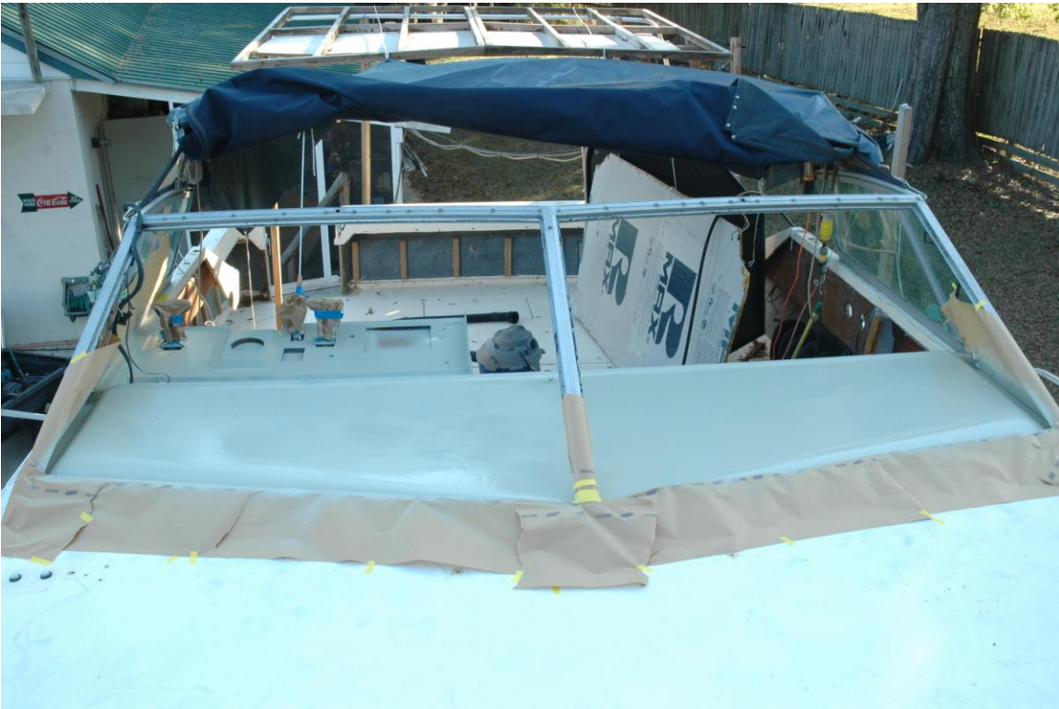
Figure 16 While the glass is out it is a good time to paint the dash and console. Also seal the windshield wiper power wires at the lower starboard corner inside the windshield. It can also be sealed from below. See the next section.
