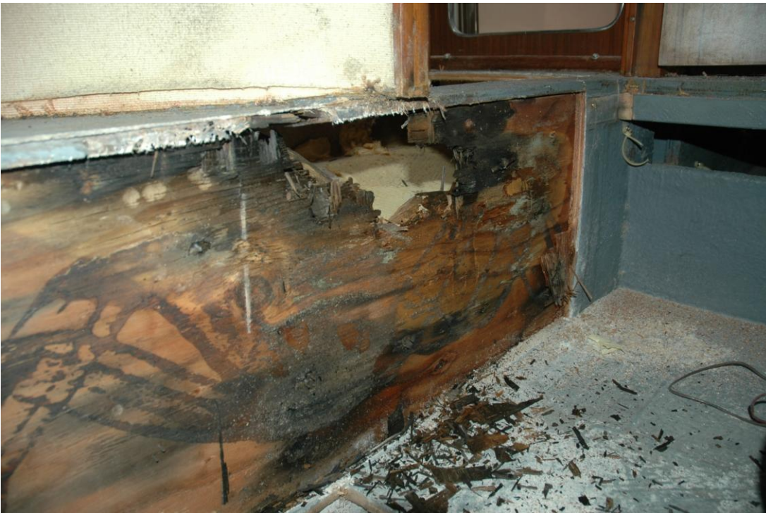
Figure 24 Rotted stringer from leaking shower or side windows.
