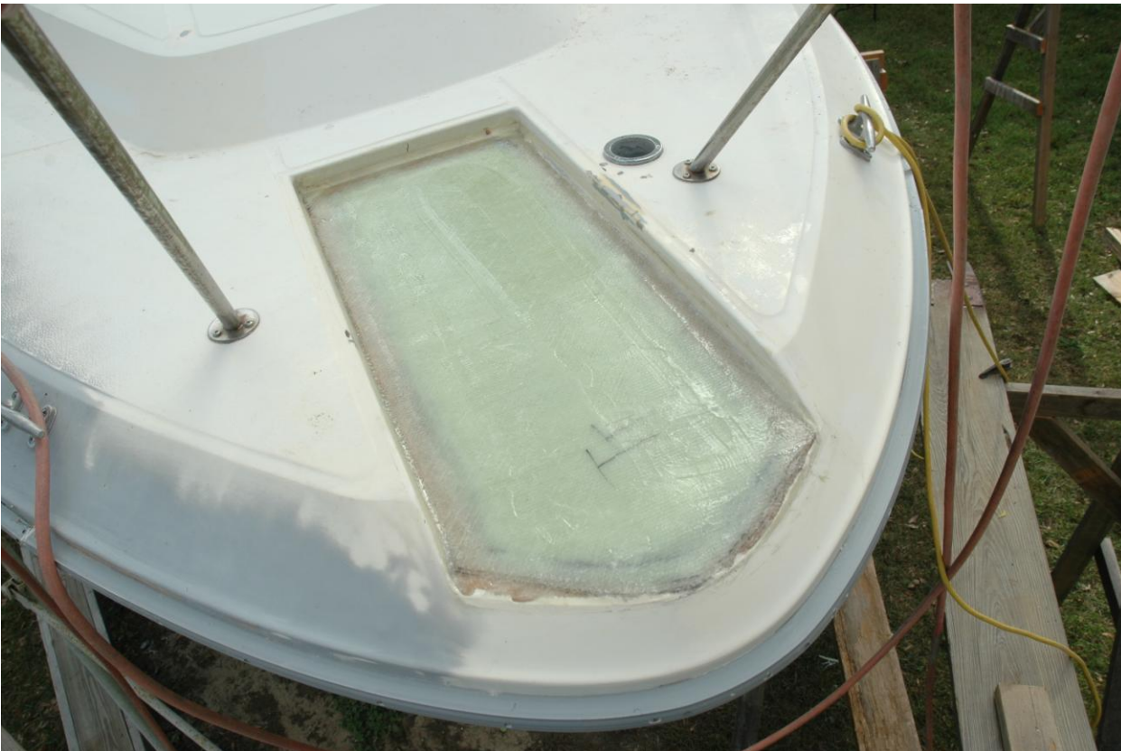
Figure 4 Replaced with solid glass and epoxy 1.5" thick
