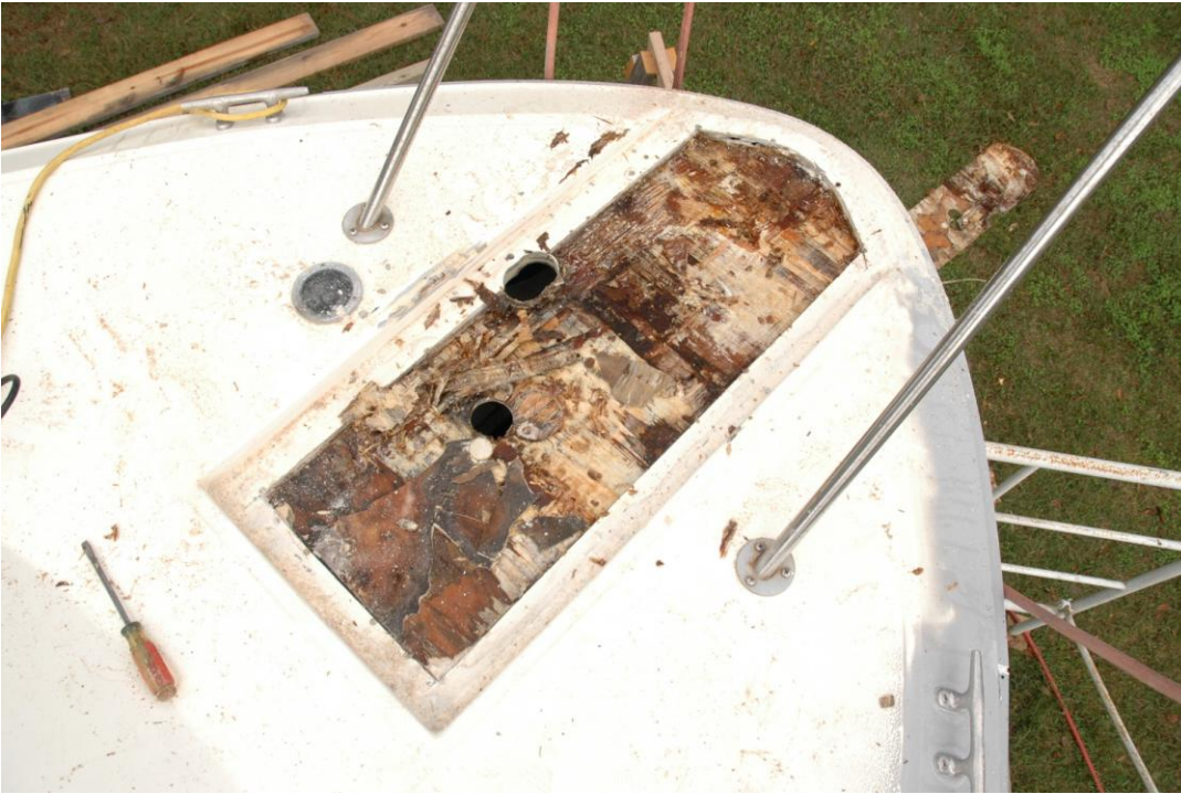
Figure 4 Replaced with solid glass and epoxy 1.5" thick
