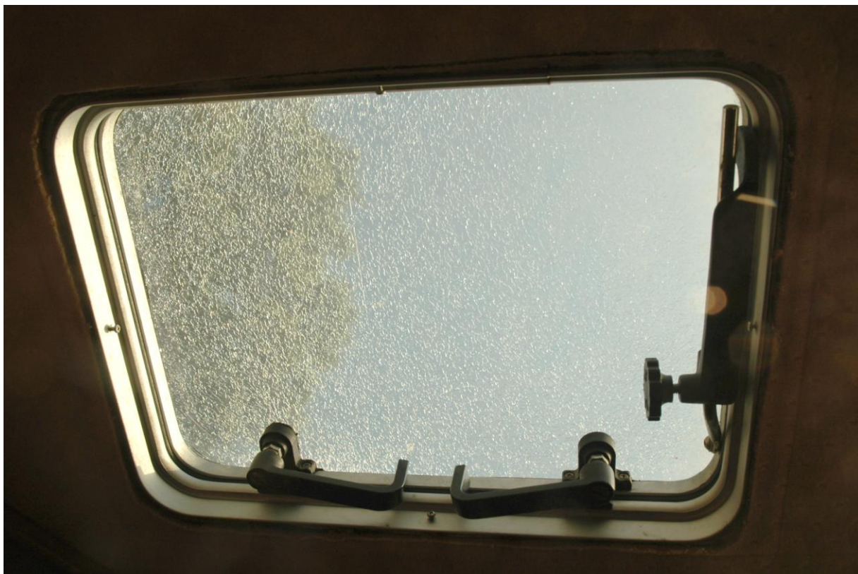
Figure 18 Might want to pull the hatch frames and seal them with 4200. They also leak. The crazing in the acrylic seems to be only cosmetic and only on the outside surface. Just looks bad.
