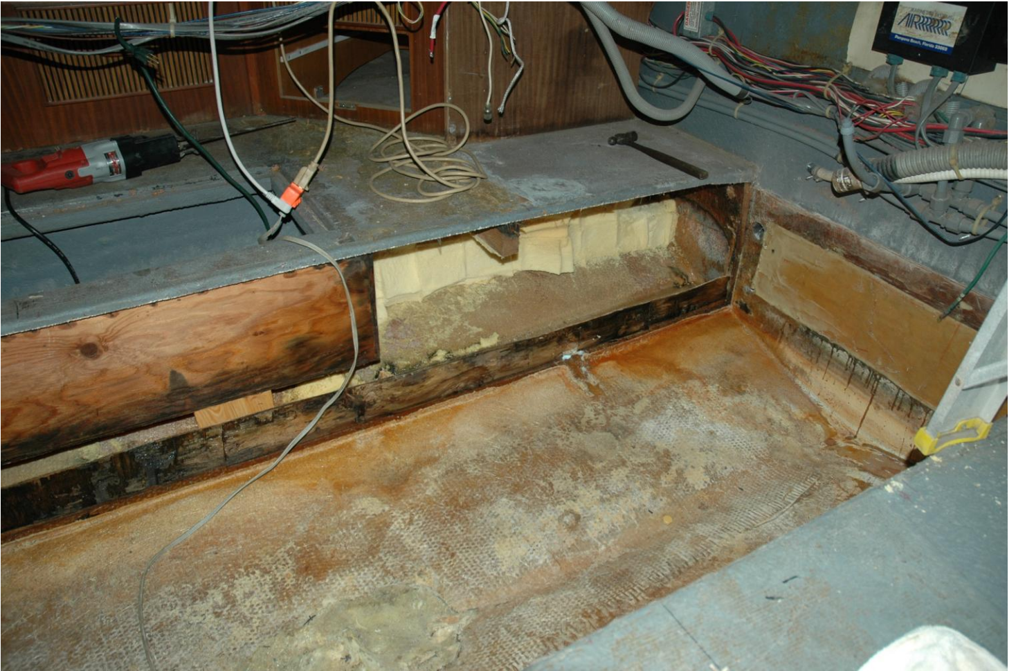
Figure 25 I cut out the stringers. They came out in handfulls of rotten wood
