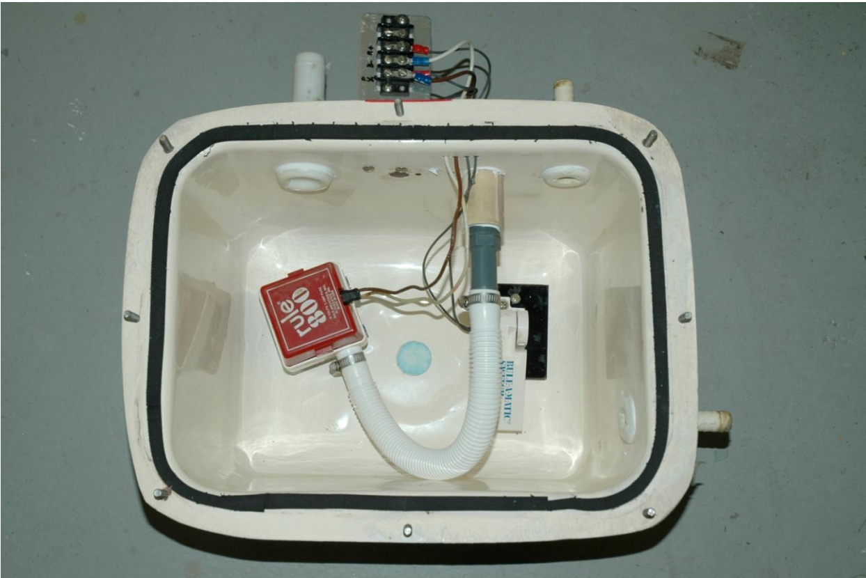
Figure 8 Shower Sump after rebuild
