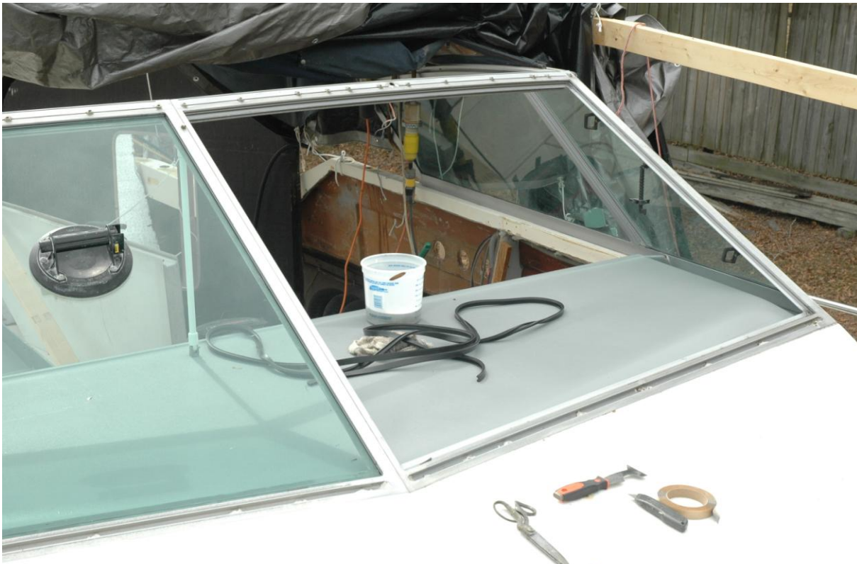
Figure 13 With a few tools it is fairly easy to R&R glass.
