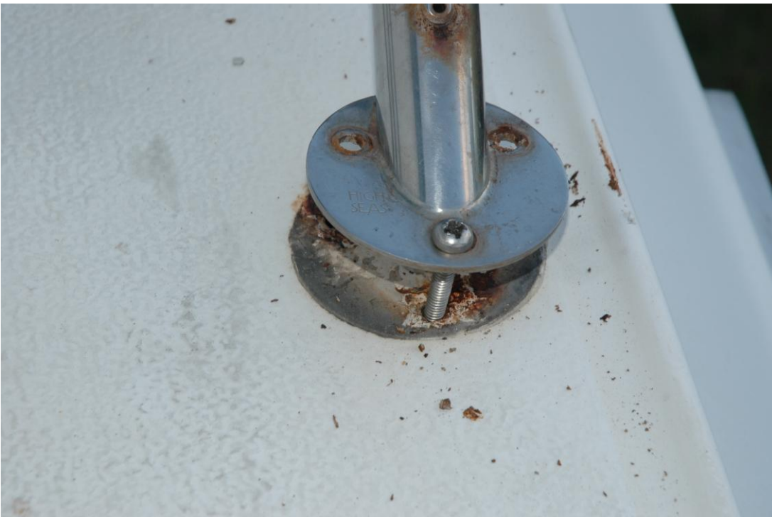
Figure 10 Stanctions have backing plates and nuts and washers below.
