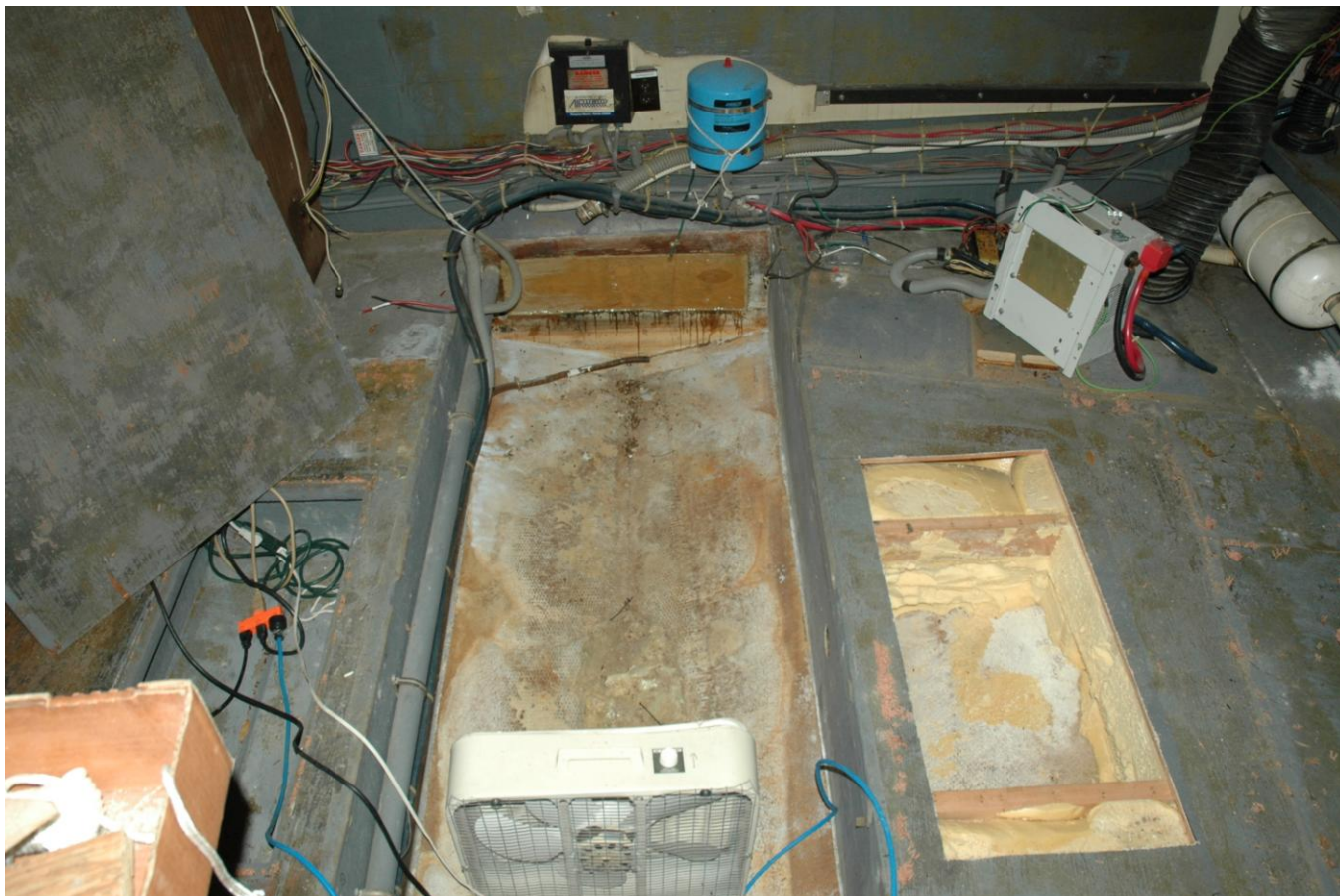
Figure 22 I pulled the floor under the tank and removed all the foam.
